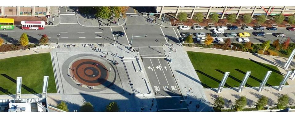
The jigsaw puzzle of 350 granite and concrete pavers were removed and replaced with a crane, and the fountain received new light stands, lenses, hoses, solenoid valves, and more. Fountain equipment in the underground vault was upgraded, as were lights in the plaza near the fountain. 156 lights were upgraded to energy-efficient color LED lights that are programmed to sync to the fountain's water shows and an incredible three miles of wire were used in the upgrades and repairs.
